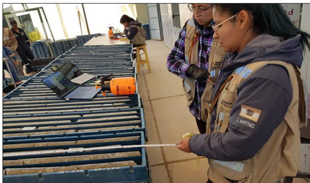
Figure 12.2 Drill Core Logging/Sampling at Iska Iska
